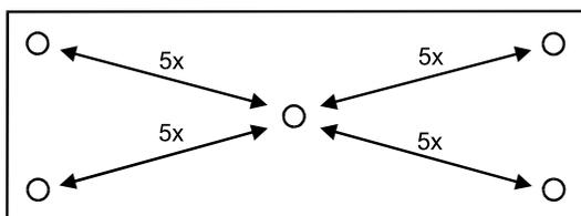
The four measurement series shall be repeated after the gauge block being rotated by 180° in the horizontal plane. The mean values and the standard deviations shall be calculated for each of the eight measurement series. The deviations  $f_o$  and  $f_u$  from the central length result from the largest and the smallest value of the eight mean values.
