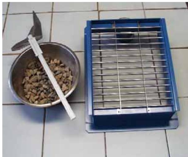
The left photograph shows piles of aggregates used for road construction. On the right are the instruments for the determination of particle shape. The bar sieve is necessary for testing according to EN 933-3, the special version of a calliper is necessary for an alternative test according to EN 933-4.
